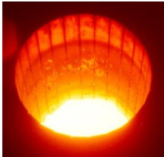
**Figure 1:** Melting of titanium in an induction furnace with cold crucible
